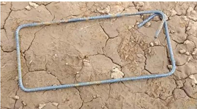
Rectangular column or rectangular beams are generally used in construction. So, we need to calculate mostly the cutting length of rectangular stirrups.
